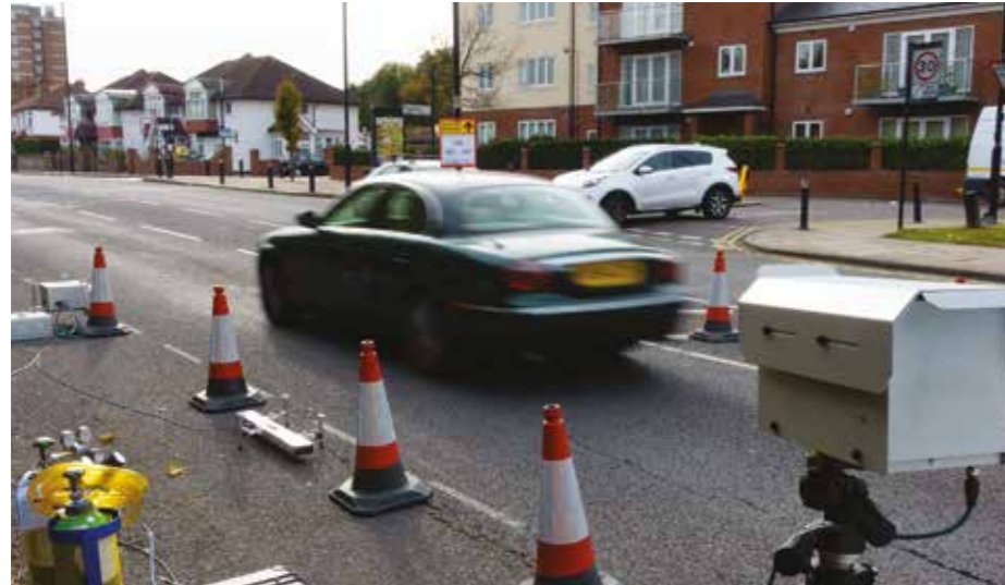
TRUE measures vehicles at random on the road, by passing a laser through the tailpipe emissions. The test is impossible to cheat.
