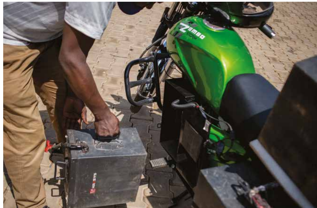
Changing a battery on a Zembo e-moto in Uganda
