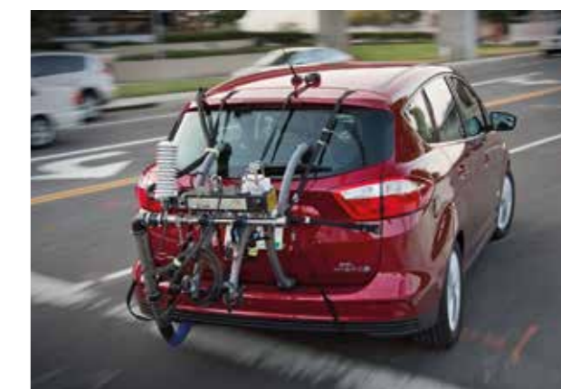
PEMS unit attached to a passenger vehicle (photo courtesy of Luca Pascotta)
