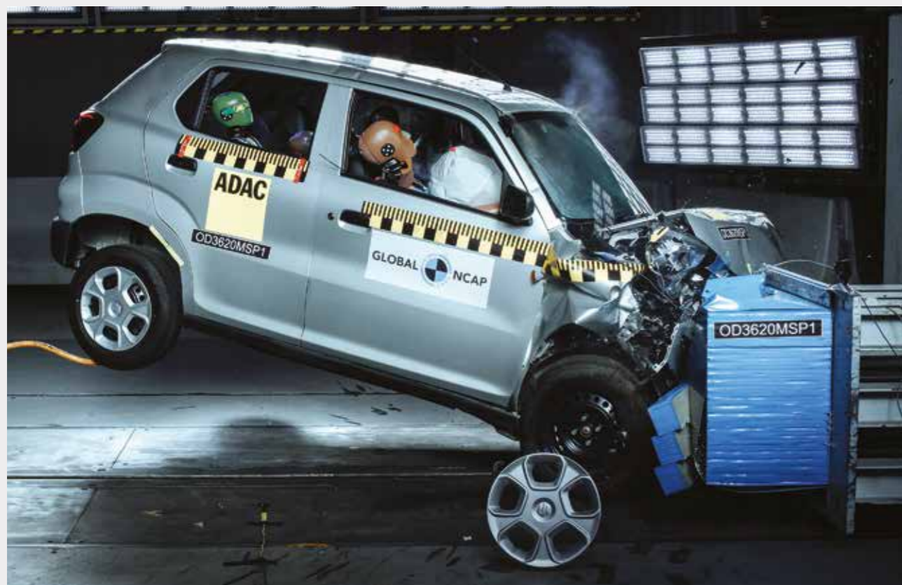
The Maruti Suzuki S-Presso achieved zero stars for adult occupant protection and two stars for child occupant protection. The S-Presso offers only a driver airbag as standard.
