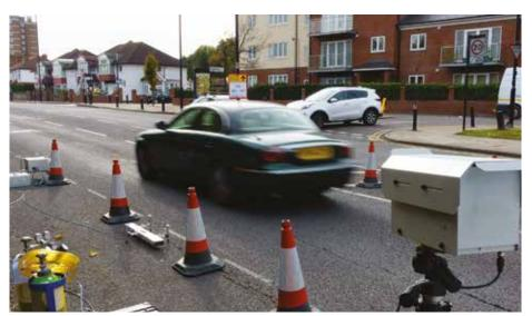
TRUE measures vehicles at random on the road, by passing a laser through the tailpipe emissions. The test is impossible to cheat.
